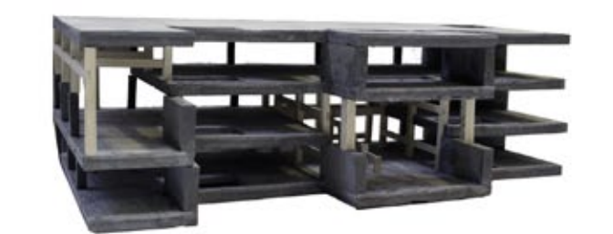
Cast Concrete test model experimenting with the placement of cuts and method of timber insertion.
